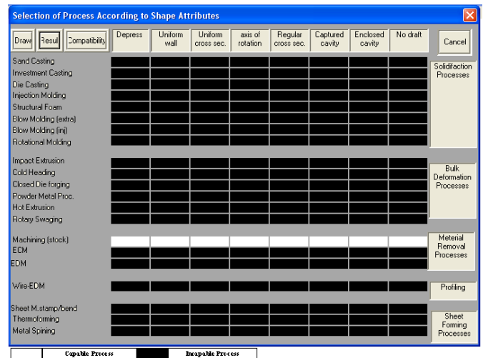
Figure (21) The capable processes for the shape attributes of the bracket part manufacturing
