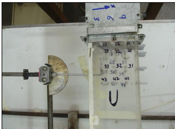
Figure (2a) Photograph shows the static pressure taps.
